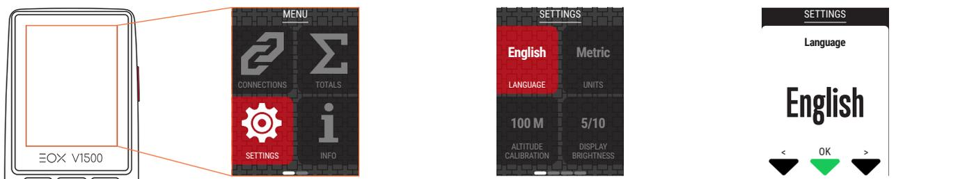
The diagram illustrates the process of setting the language on the EOX VIEW 1500 CAN display. It shows a physical device with three buttons labeled A, B, and C. The first screenshot shows the 'MENU' screen with 'SETTINGS' highlighted. The second screenshot shows the 'SETTINGS' screen with 'English' selected under 'LANGUAGE'. The third screenshot shows the 'Language' selection screen with 'English' chosen. Below each screenshot is a text box explaining the steps.
